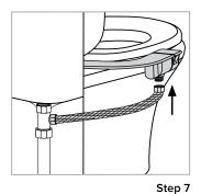
**NOTE:** If there is any leaking, check all rubber washers and make sure all water connections are tight and secure. If necessary, you can use the provided Teflon Tape (Plumber's Tape) for any leaking connections.
