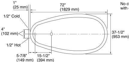
No change in measurements if connected with drain illustrated. (K-106)
