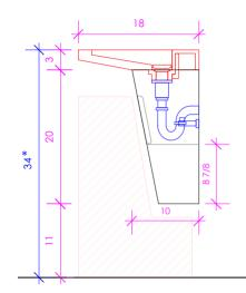
\* Recommended installation height \*\* Recommended plumbing loc
