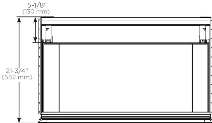
Top view for plumbing and sink clearance
