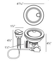
Turn the remote knob to open and close drain. Water drains easily when cover is in place. Cover flips up with easy touch. Polypropylene housing. Fits standard 3½" opening. 1¾" hole required in countertop for remote installation. Remote cable 25½" L.
